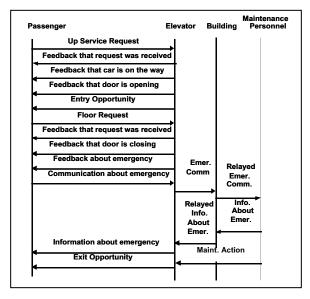
3) Passengers are receiving transportation in the elevator system when a fire breaks out in the building; building alarm system sends signal to elevator system to stop elevator cars stop at the nearest floor, provide exit opportunity, and sound a fire alarm. Passengers leave elevator cars. Elevator cars are reactivated by special access available to maintenance personnel.
